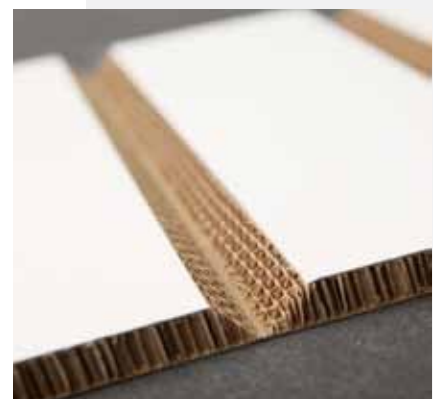
V-notch in sandwich board.
