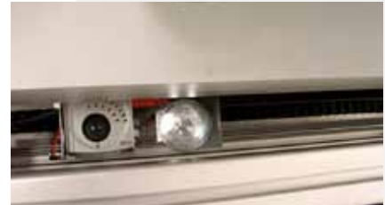
Perfect print-to-cut registration with two cameras to register marks.
