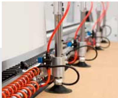
The suction grippers shake and bend the sheet to separate the material.
