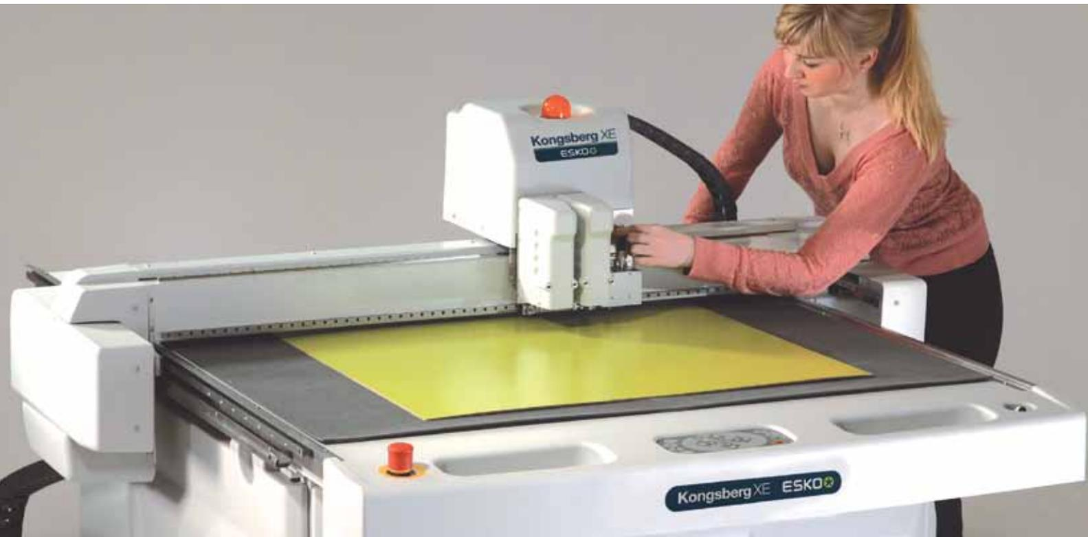
*The Kongsberg XE10 is a small-format dieless digital table for cutting and creasing folding cartons. It is based on the technology and versatile architecture of the larger Kongsberg tables, noted for their power and durability.*
